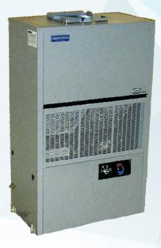
The selfcontained cooling units are specially designed for marine application and are complete with compressor, condenser, evaporator and fan built together in a casing. All electrical wiring and refrigerant piping made. To be delivered with R-407c and R-404a as refrigerant. Designed as seawatercooled.
